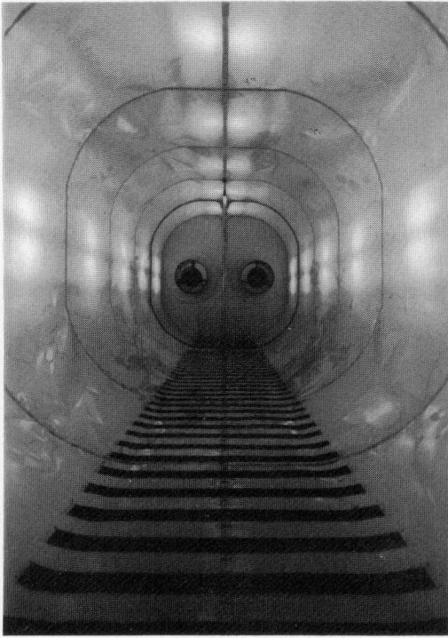
Fig. 14. Ten-meter long by 2 meter diam experimental wind tunnel built by the author to study host-seeking behavior.
