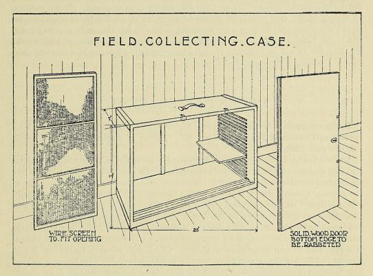
The shelves are of  $\frac{1}{4}$  or  $\frac{3}{16}$  inch wood that must be soft enough to take pins well. Five shelves to a case are ordinarily sufficient for average collecting. As shown in the cut, the cleats for the shelves do not extend quite up to the top, and when not in use for specimens the shelves can all be stowed away in the upper part, leaving the rest of the box clear for packing material and supplies, such as mouse traps, cotton, or anything not too heavy.
