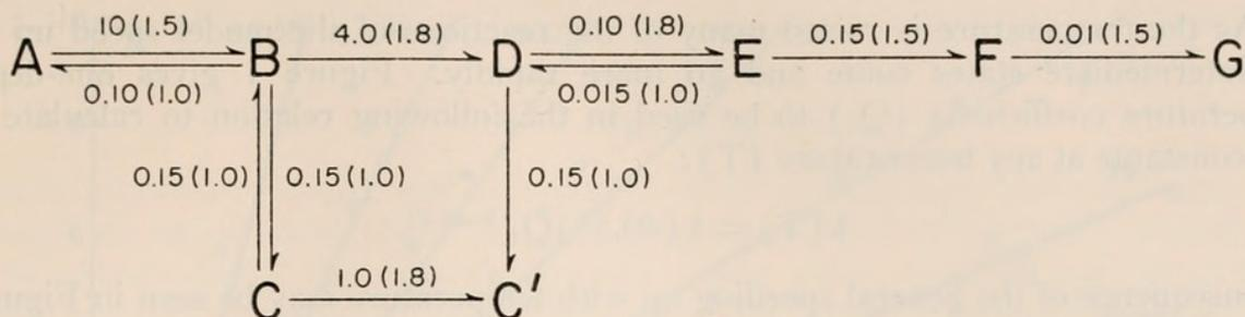
FIGURE 1. The parameters of the model. The first number by each arrow is the first order rate constant in  $\text{min.}^{-1}$  for that step. The second number, in parentheses, is the one-degree temperature coefficient,  $Q_1$ , of the rate constant.
