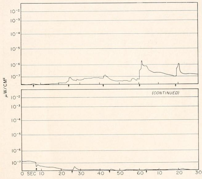
FIGURE 6. Luminescence of a single *Meganyctiphanes norvegica* when stimulated in the electrode chamber. Arrows along time scale indicate instant of stimulation. Chart speed is 6 in./min. The stimulus (0.7 amp.) was as strong as any ever used for *Metridia*. Low intensity of luminescence is notable in comparison to *Metridia's* bright flash.
