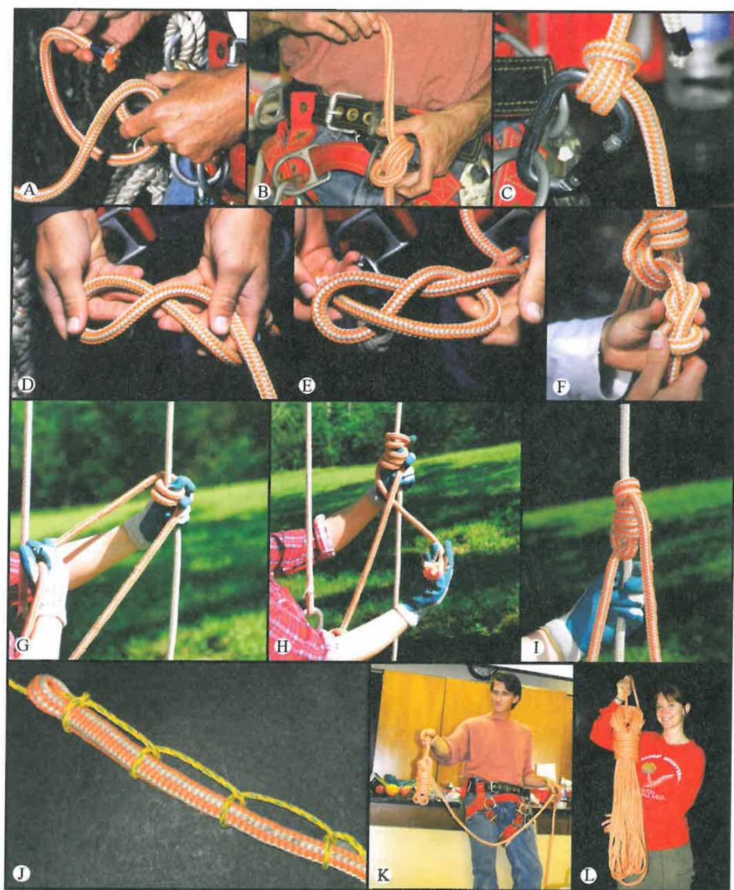
FIG. 6. A–L. Climbing knots. A–C. Anchor Hitch knot. A. Pass the working end of the rope forward over and through the carabiner twice forming two loose turns moving left to right. B. Pass the working end across the two loops from right to left then through the two loops from left to right. C. Tighten and dress the knot and add a figure eight stopper knot. D–F. Figure Eight stopper knot. D. Form the working end of the rope into a loop. Cross the working end over and under the running end forming another loop. E. Pass the working end through the first loop from the front. F. Tighten and dress the knot. G–I. Blake's Hitch Knot. G. Grab working end of rope with left hand. Use left thumb as a spacer and make four to five counter clockwise upward turns with first two or three turns over thumb. Make sure bridge between saddle and Blake's Hitch is not too long or too short. The bridge needs to be a comfortable length in a sitting position, ensure that the extra give from the climbing saddle does not lengthen the bridge to the point that the Blake's Hitch is out of reach. H. Pass the end of the split tail behind turns. Then pass the end of the split tail between bridge and working end of rope. I. Pass the end of the split tail through the lower two or three turns (depending on whether four or five total turns) held by thumb. Dress and set the knot and add a figure eight stopper knot (see F). J. Half Hitch. Pass the end of the throwline around the end of the climbing rope in a clockwise motion. Pass end of throwline over climbing rope and under throwline. Repeat Half Hitch four to five times moving down the climbing rope away from the end of rope. K. Monkey Fist. Coil 3–5 m of working end of rope. Cover the coils with several turns of rope. At end of turns form a loop and pass it through one of the loops formed by the coils. L. Gasket Hitch. Coil all but the last three to five feet of rope. While holding onto coil with one hand, make clockwise horizontal turns around the coil moving towards the head of the coil. Push a bight through and then over the head of the coil and slide bight over coil until it rests on top of the turns. Pull the end of the rope to tighten and set the knot.
