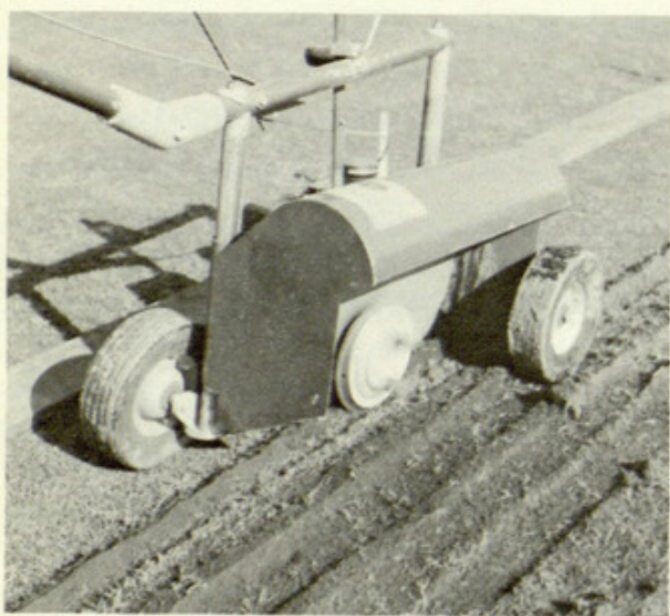
Opening trenches 1/2" wide and 6" deep with the Moist-O-Matic Mole Trencher. Accurate spacing of 6" was obtained by use of a 1" x 6" straightedge.
