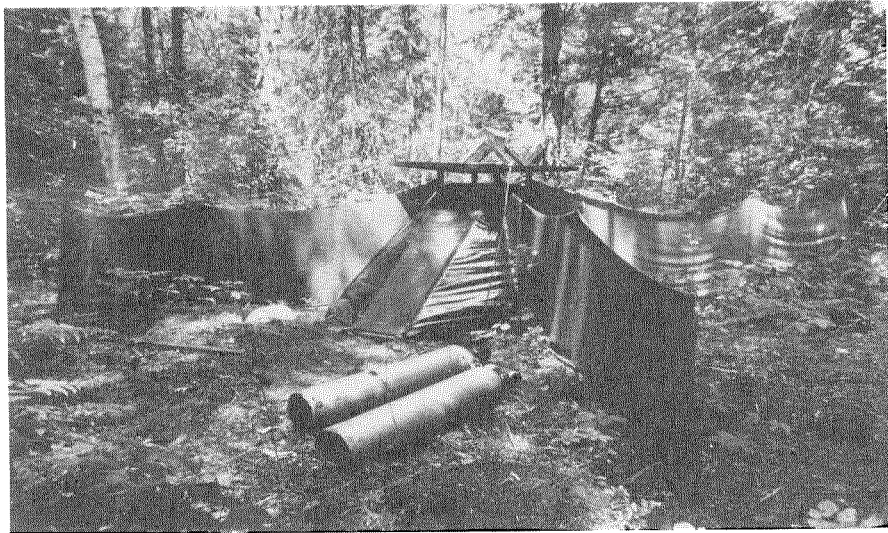
Fig. 1. Photograph of a trap in operation. Note the ramps and radiating baffles.
