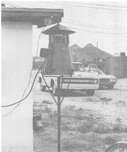
FIG. 1. Light trap bracket close-up of telescoping shaft.
