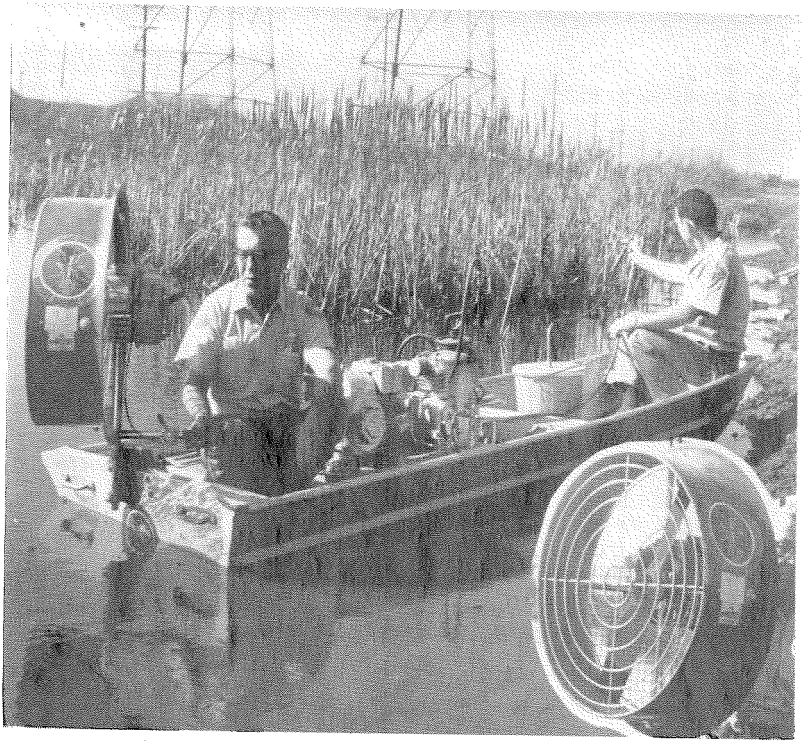
FIG. 1.—Orange County air boat in operation. Photograph shows the 24-inch McBride Air-Thrust Portable Power Unit mounted on a 12-foot aluminum pram, together with compressor and spray equipment. Inset shows partial front view of air thrust unit.
