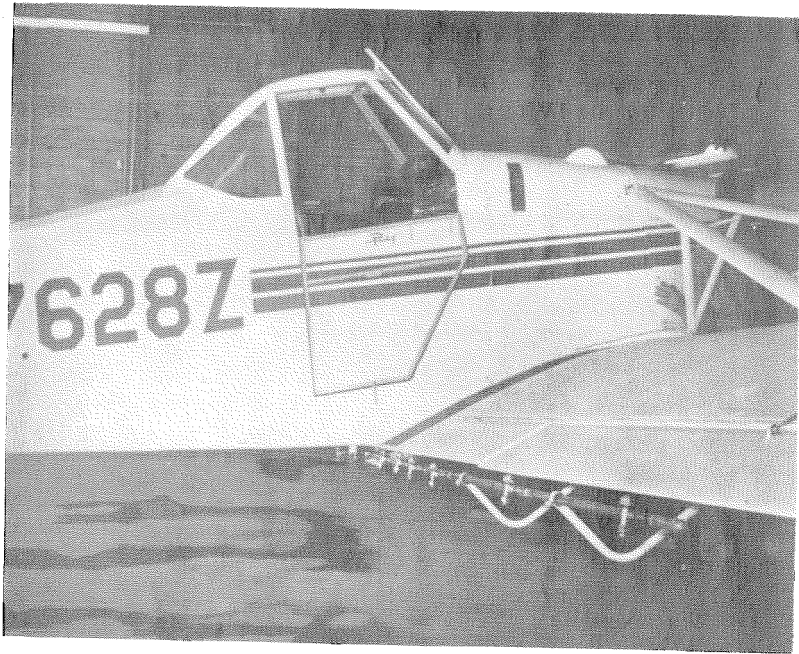
FIG. 1.—Piper Pawnee 235 fitted with 25 foot, \frac{3}{8} inch trailing-edge low volume spray boom.
