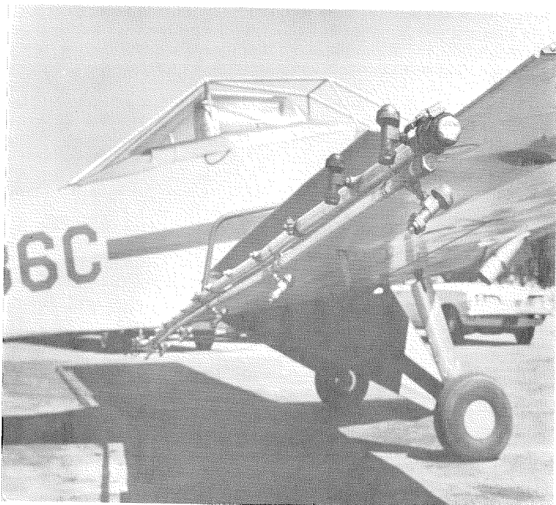
FIG. 1.—150 hp Call-Air plane supplied by Tulare Mosquito Abatement District, showing special boom of \frac{1}{2} " tubing used in low-volume applications.
