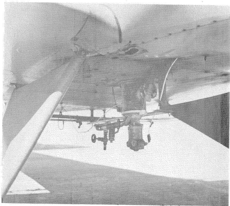
FIG. 2.—Electrically driven pump and 12 volt d.c. motor mounted on dump-valve door of Call-Air 150 hp plane used in tests in Tulare and Kings mosquito abatement districts.
