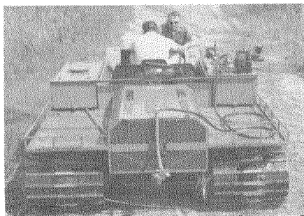
FIG. 1.—Thiokol Spryte with pump and tank, adapted for larviciding.
