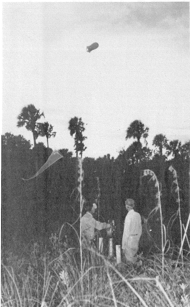
FIG. 3.—Kyttoon net for upper-air sampling of mosquito exodus.
