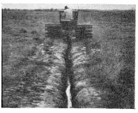
Effective clearage shows plainly in the wake of the tractor-driven "plough." Note how tractor treads crush debris flat along the bank, climinating danger of reclogging. The apparatus cleans ditches 30 times as fast as with hand labor which, up to this year, was used for all salt marsh ditching work in Connecticut.
