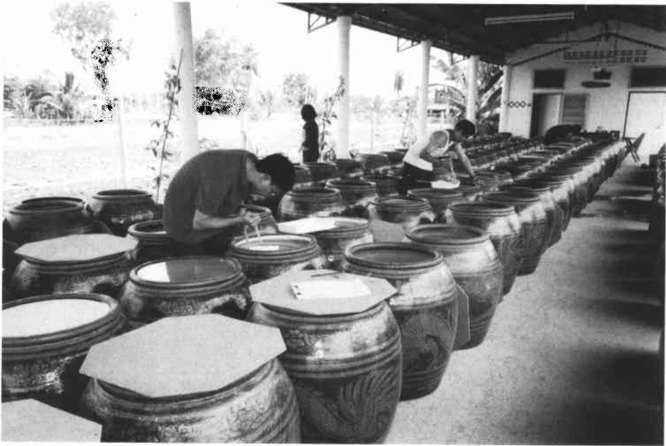
Fig. 1. Arrangement of glazed earthen jars (capacity 200 liters) for investigating the long-term efficacy of slow-release formulations of larvicides against Aedes aegypti at Bang Bua Thong, Nonthaburi Province, Thailand, in 2002.
