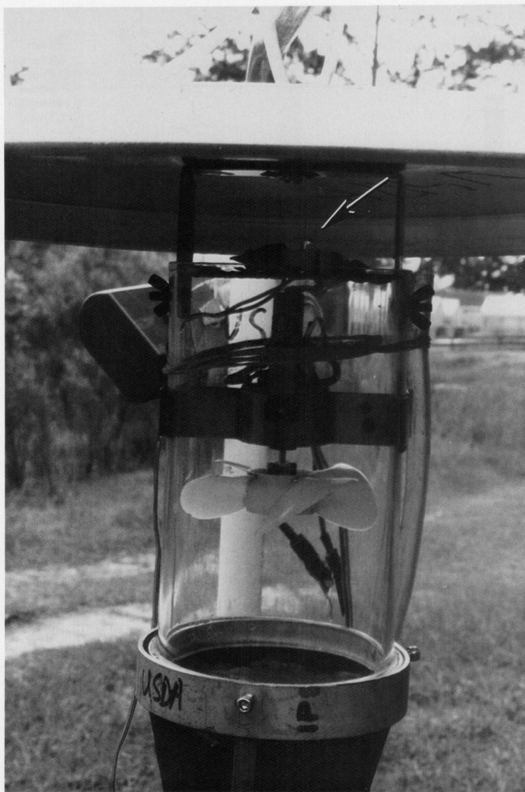
Fig. 1. Modified Centers for Disease Control (CDC)-type trap equipped with light-emitting diode (LED) (shown with arrow).
