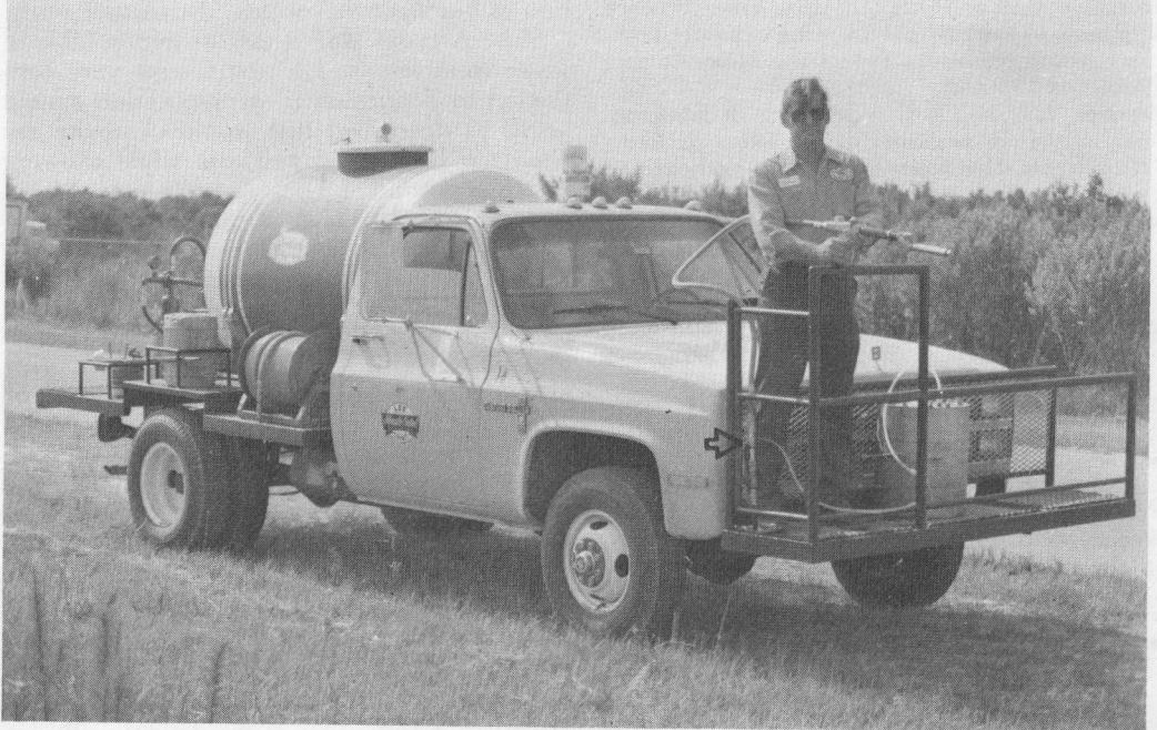
Fig. 2. Roadside ditch larviciding truck equipped with Dema injector (→).
