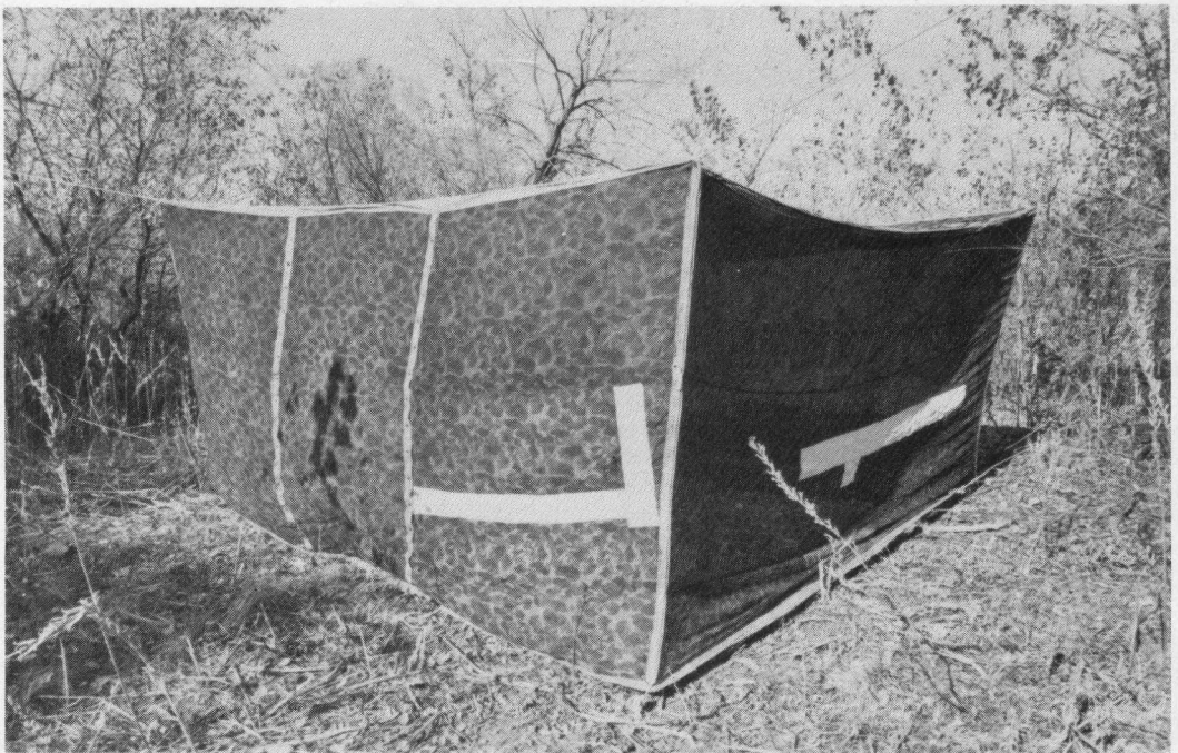
Fig. 2. Animal-baited net trap constructed of lightweight nylon tulle.
